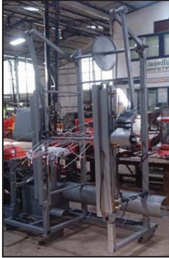
Figure 10 The primary sugarcane leaf pruning mechanism.
